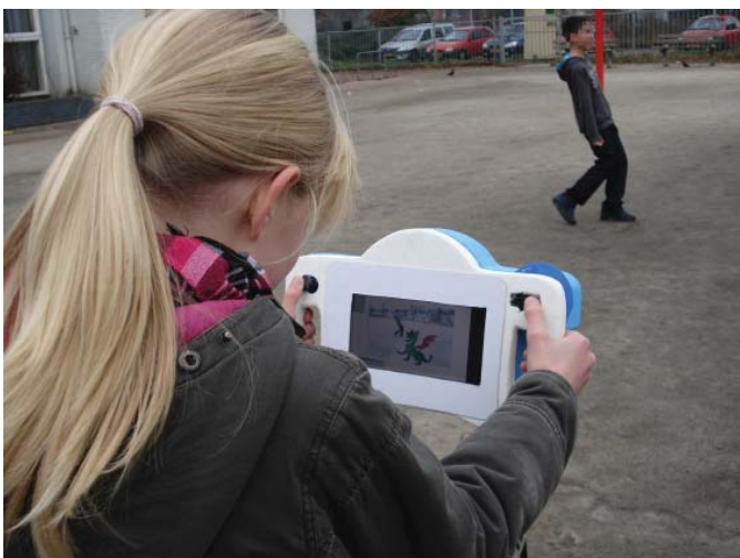
Figure 1. The final Junior Director prototype being tested at an elementary school. At the left of the device is a joystick for moving the animated character. At the right are an action button, and a dial for choosing which animated character to use.
