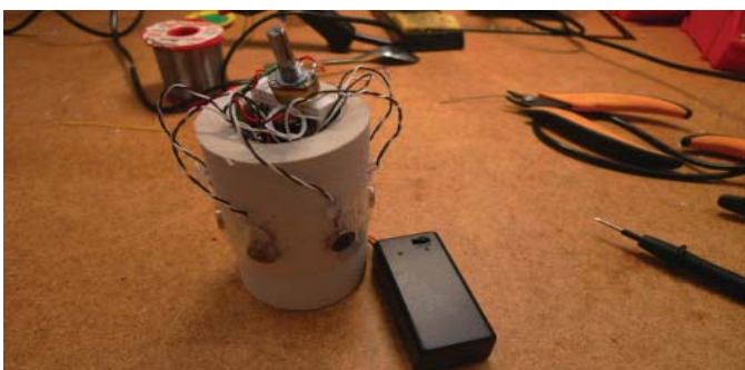
Figure 2. A grip with 7 vibrators, with manual control.
